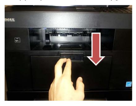
Once the manual feed tray is open, you will need to unfold the tray as shown in the picture below. To use an envelope, you will need to adjust the blue levers to fit to size.
