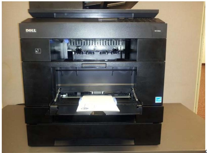
Note: For best results and to eliminate paper jams when using the manual feed tray, it is recommended to use a single envelope or sheet of paper at a time.
